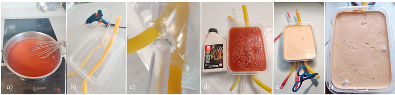
Fig 1. Gelatin homemade phantom: a) container preparation; b) several plastic tubes are placed inside and then filled with liquid; c) holes of the container are then sealed with liquid glue; d) when the jelly solidifies, a layer of liquid latex is pureed in mimicking skin; e) result after 48 hours; f) after 8 days in fridge.
